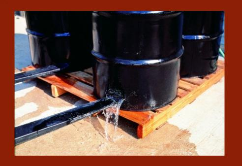
During the Phase I interview process, a site tenant reported that a forklift pierced a 55-gallon drum of xylene. Employees flushed the contents to a floor drain which is connected to an on-site septic tank and leach field.
