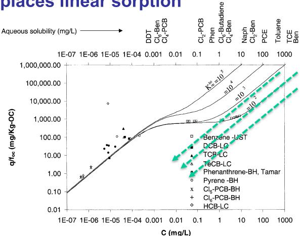
Figure: Dual Equilibrium Based Model of Non-linear sorption. Green arrows show linear isotherms; dual equilibrium model shows divergence due to non-linear sorption
