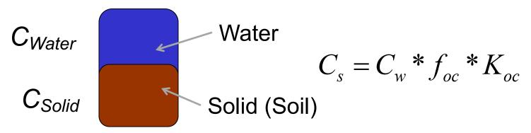
Contaminant mass will desorb from matrix into groundwater as "cleaner" groundwater migrates through system
