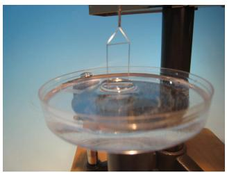
Interfacial Tension (Liquid-Liquid)
