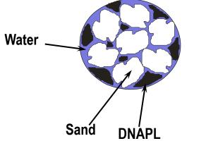
DNAPL migrates as a mobile and "continuous" body as long as the there is enough pressure (NAPL "head") to displace groundwater from the pores in the aquifer matrix.
